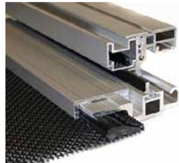
All Havengard® escape screens feature the patented 'Grip Lock' mesh retaining system. 'Grip Lock' folds and hooks the stainless steel security mesh continuously all around the window or door frame. This unique continuous extra strong interaction between the mesh and the frame means the stainless steel mesh will not pull out of the frame even after a prolonged attack.
